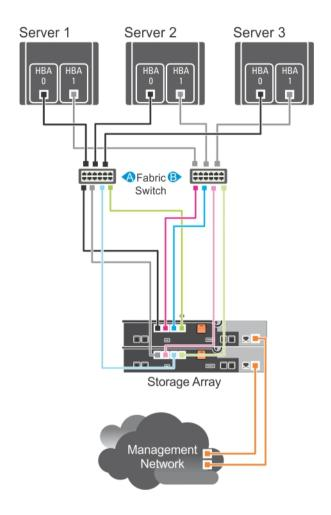
Figure 2. Three SAN-Attached Host Servers Connected to a Storage Array Using Multiple Paths
